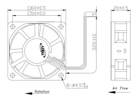
LEAD WIRES : UL 1007, AWG24, L = 320±10 mm Red = positive ; Black = negative.
