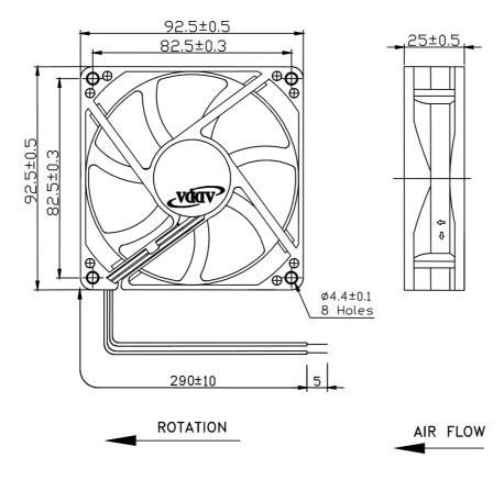
LEAD WIRES : UL 1007, AWG24 , L = 290 +/- 10 mm Red = positive ; Black = negative.
