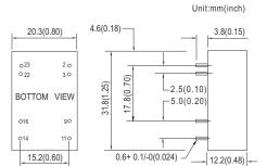
Pin Size is Tolerance  $0.5\pm0.05$ mm, Tolerance .X or .XX=  $\pm0.5$ mm
