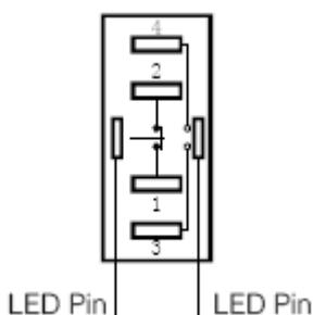
LED Pin      LED Pin      1 and 2 pin for NC, 3 and 4 pin for NO.
