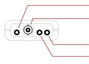
interface: connection for galv. Isolated interface adapter (accessory: GRS 3100, GRS3105 or USB3100)
