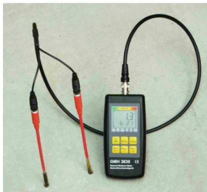
Measuring with brush probe GBSL91
