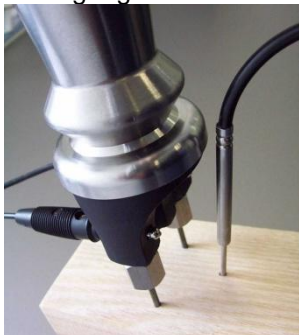
Reciprocating piston electrode GHE91 with temperature-probe GTF38
