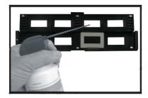
Close the slide holder and press the edges so that it locks in place.
