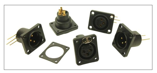
The airtight XLR is the latest XLR connector designed and made by Cliff UK. It is an airtight connector, primarily intended for applications such as active speakers, where it is detrimental to have air movement in and out of the enclosure. The movement of the speaker diaphragm can cause air pressure changes. This air can produce noise if leaked in and out of the enclosure via any small holes.
