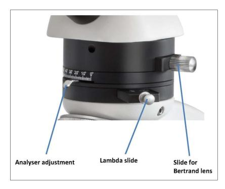
The setting of the analyser now has to be done with help of the according lever, which needs to display 0°. As a result the orthogonality between polariser and analyser, which is required for common polarisation applications, is ensured.
