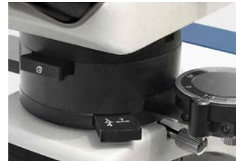
Bertrand lens, \lambda Slip, 360° rotatable analyser (detachable)
