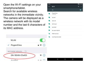
Connect your smartphone/tablet to the IP camera via the Wi-Fi connection.
