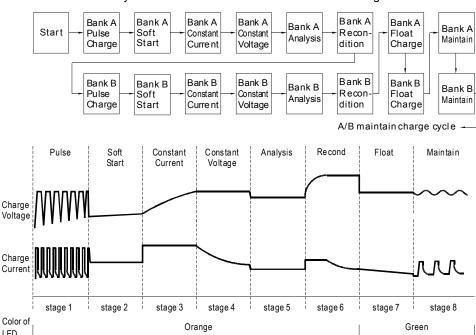
Figure 6.3 8 stage charging curve
