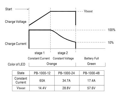
Figure 6.1 2 stage charging curve
