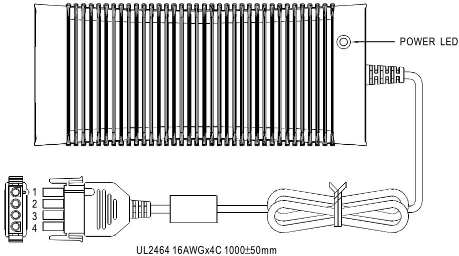
Standard male plug(power supply side): AMP 1-480702-0 equivalent
