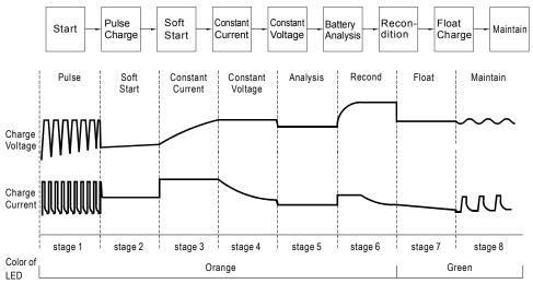
Figure 6.3 8 stage charging curve
