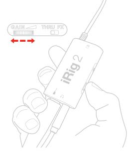
For the best sound, adjust the input level so that it's as high as possible while still retaining a "clean" sound that's not distorted or overloaded.
