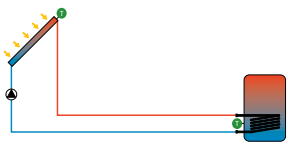
Internal heat exchanger, intelligent pump control
