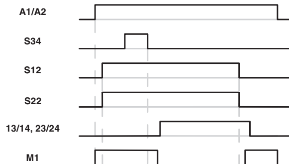
Figure 5 Time diagram for manual, monitored start
