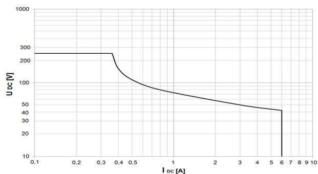
Figure 5 Relay load curve - ohmic load
