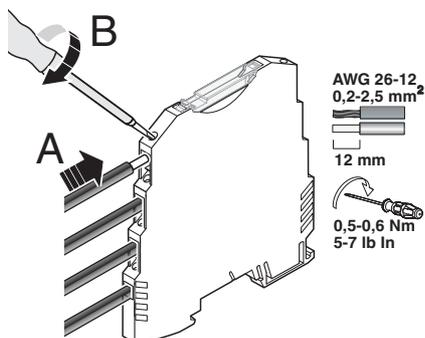
Figure 9 Connection of the cables
