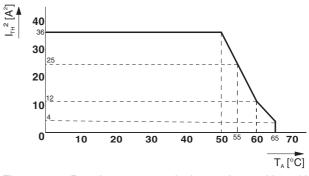
Figure 2 Derating curve - vertical mounting position with connected modules
