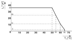
Figure 4 Derating curve - mounting position with module front at the top and aligned modules
