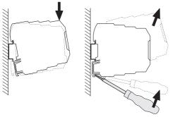
Figure 8 Mounting and removing
