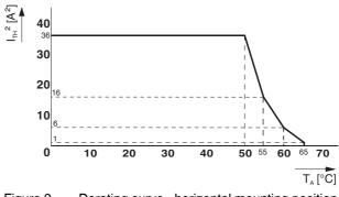
Figure 3 Derating curve - horizontal mounting position with connected modules
