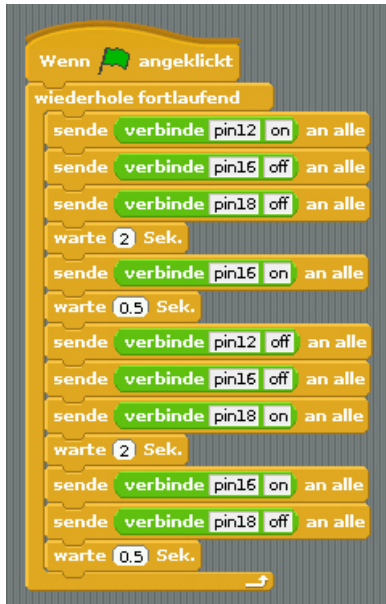
The program 03ampe1 controls the traffic light
