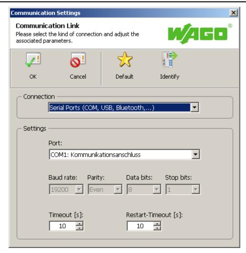
Figure 32: "WAGO ETHERNET Settings" - Communication link
