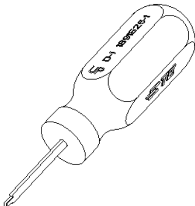
Fig.1 引抜工具(Extraction Tool)
