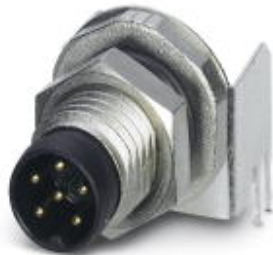
Sensor/actuator flush-type connector, plug, 6-pos., M8, rear/screw mounting with M8 fastening thread, with angled solder connection
