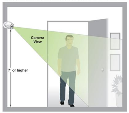
• Aim with the cloud. Use Arlo's Position mode to send video to the cloud as quickly as possible. This allows you to aim the camera while watching the video
