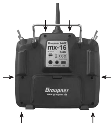
Arrangement of the case back screws
