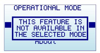
If your analyzer includes two modules (e.g. ISM Combo) only one of the modules may be the one with the available functionality. Make sure to select the right module before trying to use the functionality (e.g. the ISM Combo has the 2.4G module enabled on the SMA module at the right) otherwise above message will popup.
