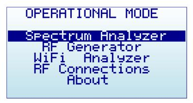
Use [Up] and [Down] arrow keys to select the desired mode and click on [Enter] to activate it immediately.
