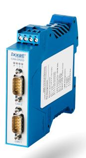
The modular CAN repeater CAN-CR200 with two CAN interfaces and one CAN backbone interface can be used to improve the load capacity of the CAN bus with nodes, to establish a physical coupling of CAN bus systems or to insert a galvanic isolation.
