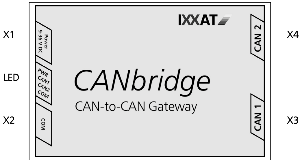
Fig. 2-1: Pin allocation aluminum version
