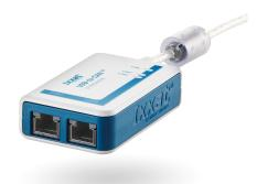
The Ixxat USB-to-CAN V2 professional with two CAN channels and galvanic isolation is an super versatile, uncomplicated and cost-efficient way to connect a computer to two CAN bus networks and is a very reliable workhorse for CAN applications e.g. in the field of test, development, maintenance or control applications.
