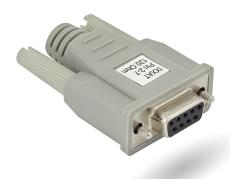
These connectors provide easy and quick termination to any high-speed CAN/CAN FD product. The connectors are used when a CAN node without internal terminal needs to be terminated or if no CAN node is connected at the end of the CAN bus. According to ISO 11898-2, high-speed CAN buses/systems must be terminated at their ends by resistors.
