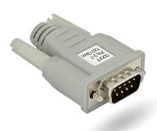
These connectors provide easy and quick termination to any high-speed CAN/CAN FD product. The connectors are used when a CAN node without internal terminal needs to be terminated or if no CAN node is connected at the end of the CAN bus. According to ISO 11898-2, high-speed CAN buses/systems must be terminated at their ends by resistors.
