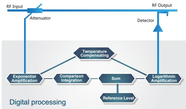
Enhanced protection circuitry on the DSG800 RF output limits reverse power and DC signals that could damage the instrument. In addition, all interfaces adopt anti-static measures to minimize damage due to static discharge. The DSG800 also features a no-wear electronic attenuator. This all electronic design is superior to a mechanical attenuator because the output level will remain stable and as-set, even if an application requires frequent level switching.
