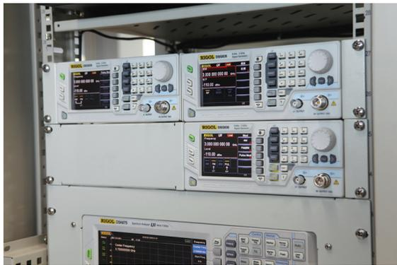
In addition, the DSG800 is designed with a standard height of 2U and half cabinet width which saves rack space. The rack mount kit not only provides side-by-side installation mode, but also vertical parallel installation mode which will reduce the line length and complexity in application fields (such as intermodulation distortion) that require more than one RF source.
