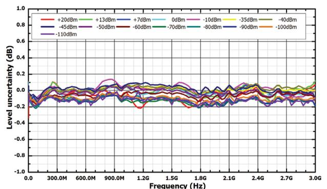
Output power with accuracy is another excellent performance feature of the DSG800. With a maximum output power of + 20 dBm (typical) and an amplitude accuracy of 0.5dB (typical), the DSG800 is perfect for
