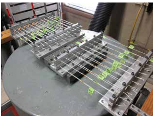
Figure 2 – Military Vibration Test - SOLISTRAND Splices
