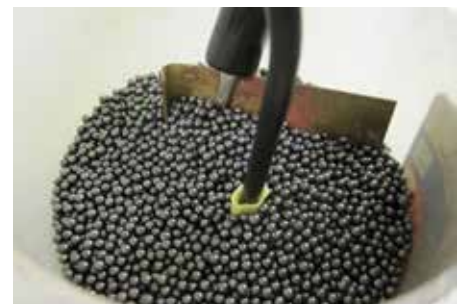
Figure 6 – Dielectric Strength Test - PLASTI-GRIP Terminal
