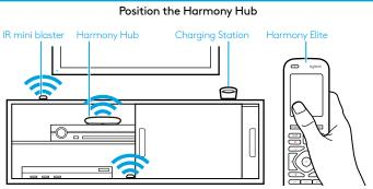
The Harmony Hub can be placed in any unobstructed location where IR signals can be transmitted to AV equiment or it can be placed behind closed cabinets with the IR mini blaster transmitters connected to the hub and positioned as shown above.
