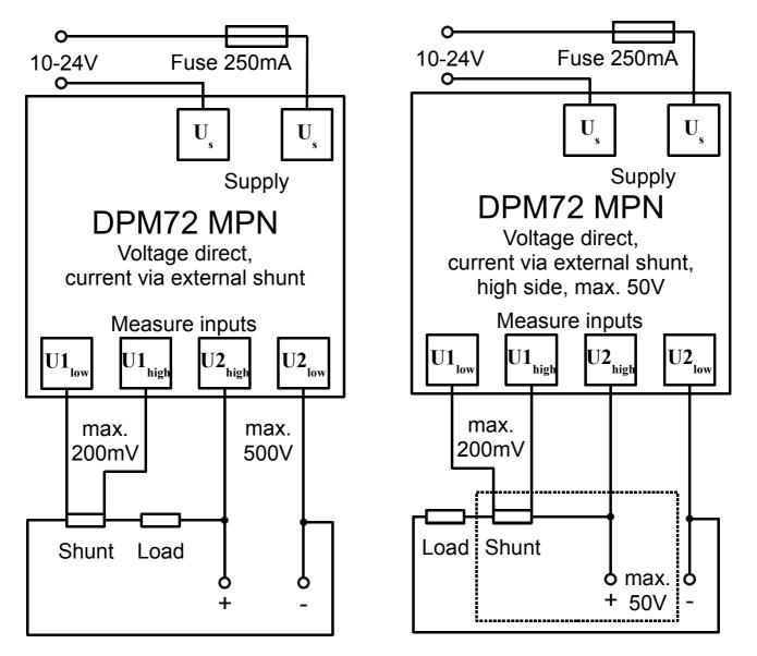
Warning: Voltage measurement on the high side (between plus and load) is recommended only for voltages up to 50V!
