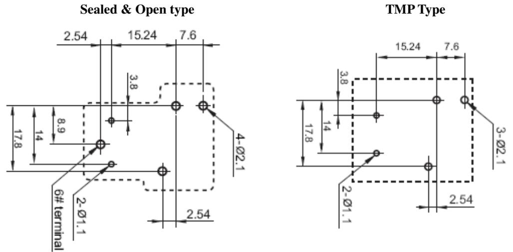
**Remark:** 1) In case of no tolerance shown in outline dimension: outline dimension  $\leq 1\text{mm}$ , tolerance should be  $\pm 0.2\text{mm}$ ; outline dimension  $> 1\text{mm}$  and  $\leq 5\text{mm}$ , tolerance should be  $\pm 0.3\text{mm}$ ; outline dimension  $> 5\text{mm}$ , tolerance should be  $\pm 0.4\text{mm}$ .
