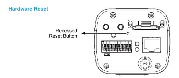
The reset button is used to reset the system or restore the factory default settings. Sometimes resetting the system can return the camera to normal operation. If the system problems remain after reset, restore the factory settings and install again.
