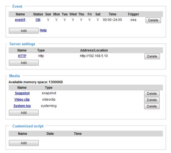
When the Event Status is **ON**, the event configuration above is triggered by motion detection, the Network Camera will automatically send snapshots via e-mail.
