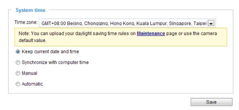
Keep current date and time: Select this option to preserve the current date and time of the Network Camera. The Network Camera's internal real-time clock maintains the date and time even when the power of the system is turned off.
