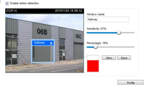
The Percentage Indicator will rise or fall depending on the variation between sequential images. When motions are detected by the Network Camera and are judged to exceed the defined threshold, the red bar rises. Meanwhile, the motion detection window will be outlined in red. Photos or videos can be captured instantly and configured to be sent to a remote server (Email, FTP). For more information on how to configure an event setting, please refer to Event settings on page 106.
