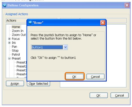
3. The Assigned Action will appear beside Button 1 in the right column as shown in the following diagram. Note that a button can only be assigned with an action. If you want to modify the settings, select the action on the list and click **Clear Selected**.
