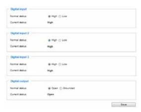
Connect DI or DO devices to the camera's terminal block, the camera will automatically detect the current connection state as pulled-high or pulled-low. You may then define the triggering condition.
