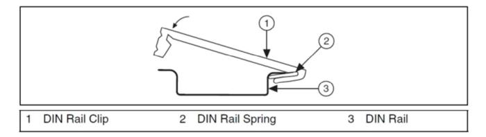
Figure 1. DIN Rail Clip Parts Locator Diagram
