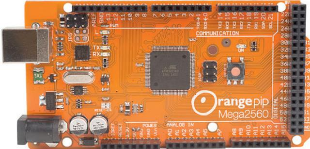
**External Interrupts: 2 (interrupt 0), 3 (interrupt 1), 18 (interrupt 5), 19 (interrupt 4), 20 (interrupt 3), and 21 (interrupt 2)** These pins can be configured to trigger an interrupt on a low value, a rising or falling edge, or a change in value. See the `attachInterrupt()` function for details.
