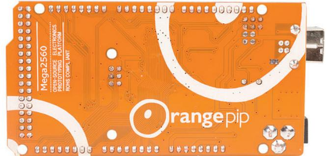
is 160 mil (0.16"), not an even multiple of the 100 mil spacing of the other pins.
