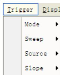
The trigger determines when the oscilloscope starts to acquire data and display a waveform. When a trigger is set up properly, it can convert unstable displays or blank screens into meaningful waveforms.
