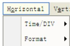
1. **Time/DIV**: leads the setting of the time base parameters
