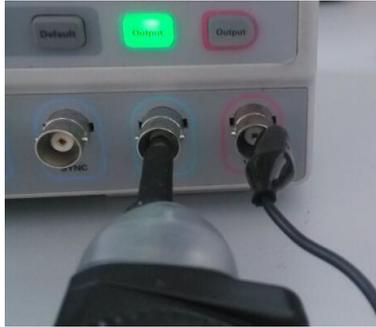
1. Attach the tip of probe and ground nip to the Connector of Probe. A square wave will be displayed within a several seconds. (Approximately 1 kHz, 2V, peak- to-peak).
