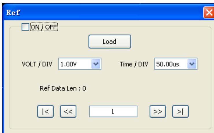
You can change the vertical scale of a waveform. The waveform display will contract or expand relative to the reference level.
