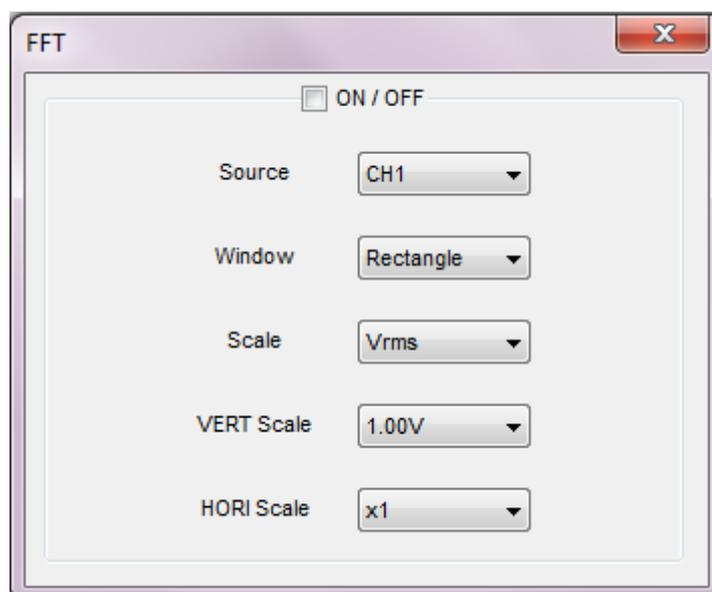
You can select the Source channel, Window algorithm, FFT number, and FFT Zoom factor. It displays only one FFT spectrum at a time.
