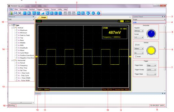
In addition to displaying waveforms, the display area is filled with many details about the waveform and the oscilloscope control settings.
