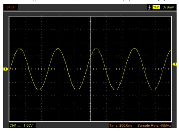
If the **Dots** type mode is selected, the waveform will be displayed as following figure.
