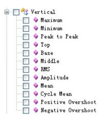
Maximum: Voltage of the absolute maximum level, Measured over the entire waveform
