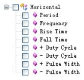
**Period**: Time to take for the first signal cycle to complete in the waveform
