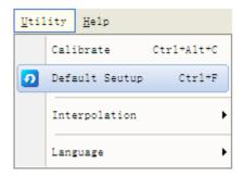
When you click the **Default Setup** in **Utility** menu, the oscilloscope displays the CH1 waveforms and removes all other waveforms.
