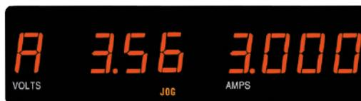
Voltage and current can be read on the main display at the touch of a button. An independent output on/off switch is provided.
