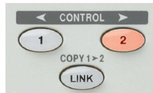
For even greater flexibility, the outputs can be linked when set to different voltages or currents allowing separate settings to be loaded into the linked-mode memories for simultaneous recall.
