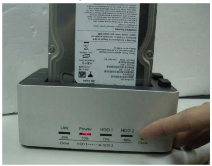
Following light-on of all 4 LEDs in orange, LEDs will then proceed to running back & forth indicating the clone progress. Each orange LED refers to every 25% of clone completion. It is only when every 25% of HDD1 is cloned to HDD2 that such LED will remain constantly on, leaving the other LED(s) in running stage. When Clone operation is fully completed, all LEDs will flash regularly in orange color until the device is power cycled.
