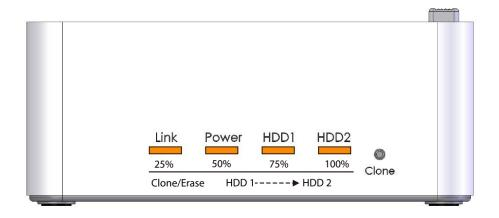
**NOTICE:** Any time clone operation fails, LED on HDD2 flares in red, leaving the other LEDs off. Refer to Section 4.4 & 4.5 in "Normal & Clone Mode Table Chart" under "Diagnosis of LED" in below "NOTE" session for details.
