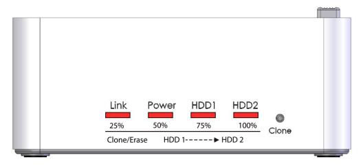
**NOTICE:** Percentage of Erase completion attributes to erasing all sectors of the inserted HDD(s). For example, total no. of sectors for two 3TB HDDs is double
