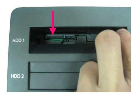
STEP2: Install either 2.5" and/or 3.5"HDD/SSD(s) to the docking station and connect to the SATA connector(s) well.
