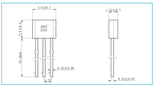
Note: In the package outline figure, Pin 1 is Vcc, Pin 2 is GND, Pin 3 is output
