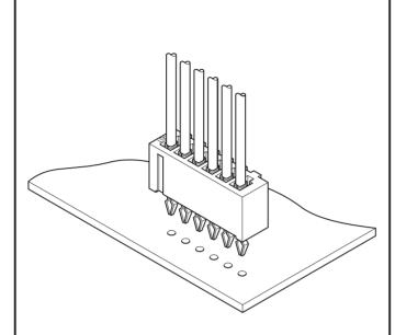
This 2.5mm pitch multi-circuit board-in connector meets the needs for high-density mounting on printed circuit boards efficiently and economically. The connector can be used for VCRs, car stereo systems, audio products, and many other consumer-oriented electronic products.
