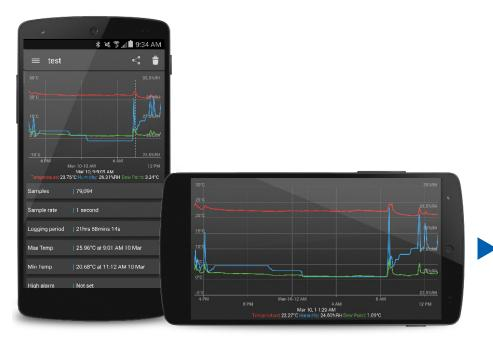
View logged temperature, humidity readings and calculated dew point, minimum and maximum values, and alarm breaches. Use zooming and panning features to view critical data with ease.
