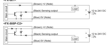
Note: The quick-connection sub cable does not incorporate +V (brown) and 0V (blue). The power is supplied from the connector of the main cable.
