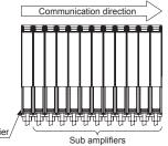
• When this product and other products (e.g. fiber sensor amplifiers, pressure sensor controllers, etc.) are connected together in cascade, install those products so that they are in order of Group A, B, D and C as shown in the right figure. This product is included in Group D.
