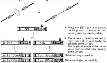
ote: The shift value of approx. 15% is an initial value. Display of the shift value can be changed to percentage [approx. 0 to 999% (unit 1 %)] or incident light intensity [0 to 9999 (unit 1)]. For setting the shift amount, refer to "PRO MODE OPERATION MANUAL."
