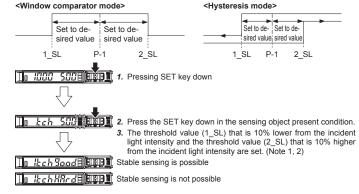
Notes 1) The shift amount of 10% is an initial value. The shift amount can be set in PRO mode. Furthermore, the shift value can be set in incident light amount. For setting method, refer to "PRO MODE OPERATION MANUAL."
