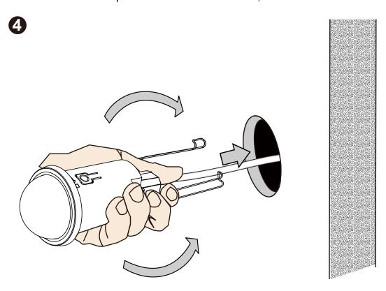
5. The retention clips will hold the module in place.
