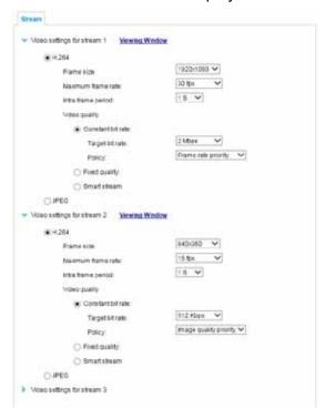
This Network Camera offers real-time H.264 and MJPEG compression standards (dual Codec) for real-time viewing.
