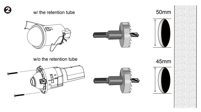
Use the M3 self tapping screws if installed without the retention tube. Note that this type of installation does not apply to hard surfaces, such as a concrete wall.
