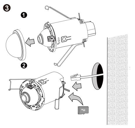
4. Pull the retention clips to the back of the camera, and then insert the camera into the wall.
