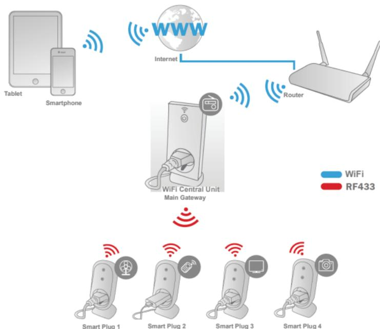
\* Please make sure that the WiFi Central Units and Smart phones are connected to Internet in order to install and control POWER ON/OFF via Smart Phone anytime anywhere.
