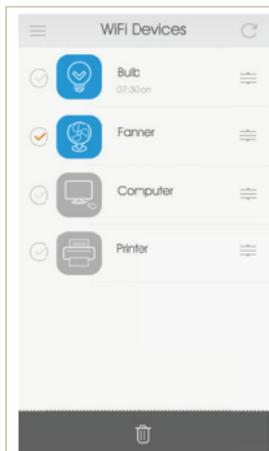
(4) Long press the device icon on the APP, then you can delete the device by selecting the desired one and press the bin icon to "Delete".
