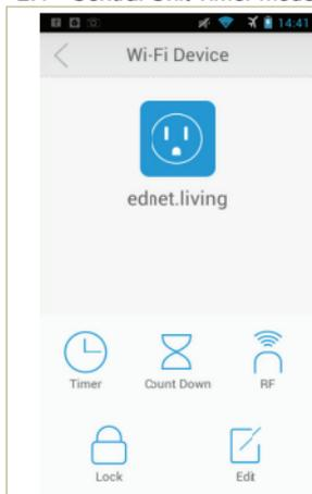
(1) Click the device icon on "WiFi device" list, the control interface will show 6 options. The Timer is the setting to control the WiFi Central Units ON or OFF under defined clock time.
